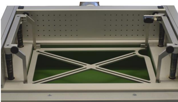
Immersion bath with 2 stepper motors, stencil holder and optional U-suction
